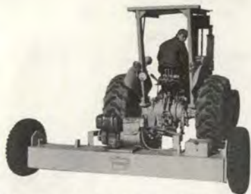
Seymour Johnson's electro-magnet has prevented many FOD incidents.
